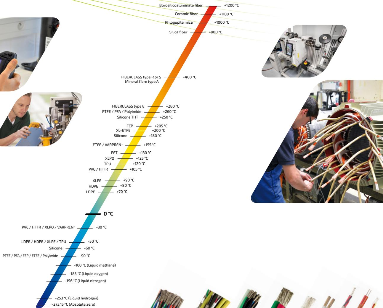
Cryogenic temperatures: In this range, only fluorinated insulations (ETFE, FEP, PFA, PTFE) or polyimide insulations retain their mechanical properties. They can therefore be used as insulations, under certain conditions. For more information contact us.
